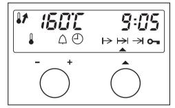
■ Call up the → symbol for duration by turning the function dial (right hand dial) until the triangle is underneath the middle arrow.
